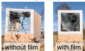
Glass scattering behavior (Protective effect of film) Ref: Report on technical standard for explosion mitigation of explosives (2021)
