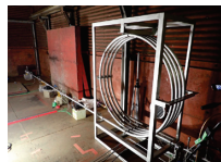
Experimental equipment for extinguishing detonating flames that propagate long distances in pipes (the Artificial Photosynthesis Project (ARPCHEM) of the New Energy and Industrial Technology Development Organization (NEDO))
