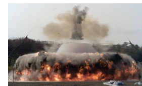
Detonation of ANFO Explosive (from report on technical standard for explosion mitigation of explosives (2016))
