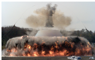
Detonation of ANFO explosive Ref: Report on technical standard for explosion mitigation of explosives (2016)
