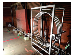
Experiments of extinguishing detonating flames that propagate long distances in pipes (the Artificial Photosynthesis Project of NEDO)
